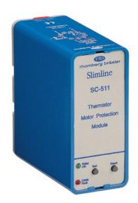
The Rhomberg Electronics SC510 and SC511 Thermistor Motor Protection modules interface with Thermistor (PTC) as per DIN 44081 which detect overheating of equipment such as motors, alternators and transformers. The Slimline SC510 and SC511 offer a failsafe feature and have sensor and cable fault detection which means that if either a short circuit or an open circuit is detected, the relay is de-energised. They also provide LED indication of both relay and cable fault status.
